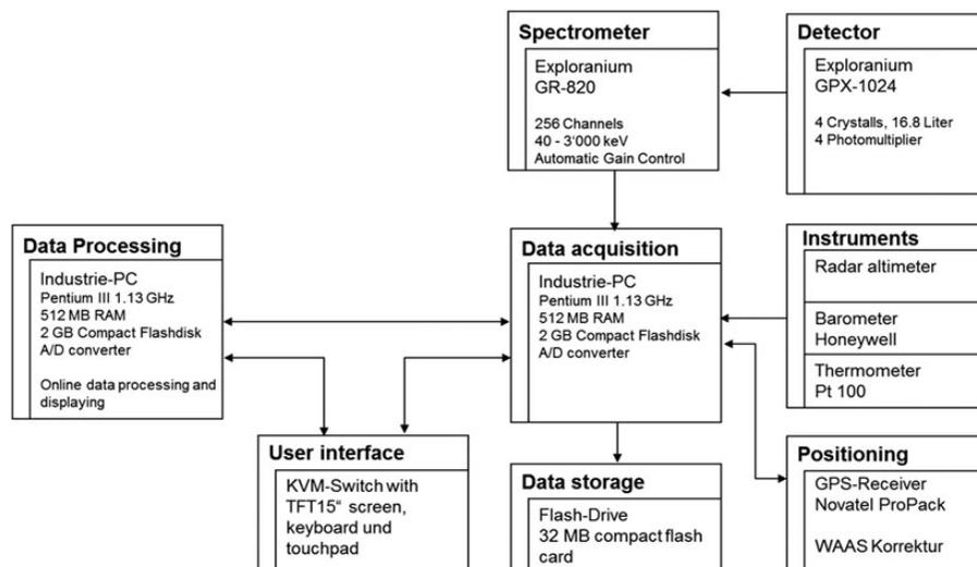
Figure 1. Schematic view of the Swiss measurement equipment.
