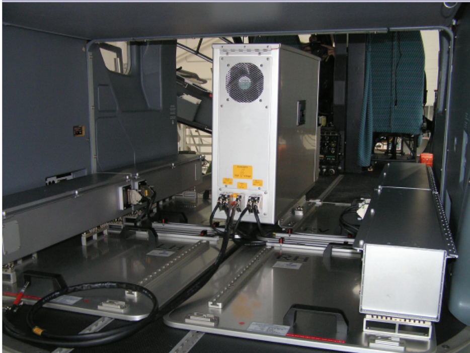
Figure 6: The German measuring system installed in the cargo bay of an Eurocopter EC135 helicopter. Right and left side: NaI(Tl)-Detectors. Center: Data processing unit.
