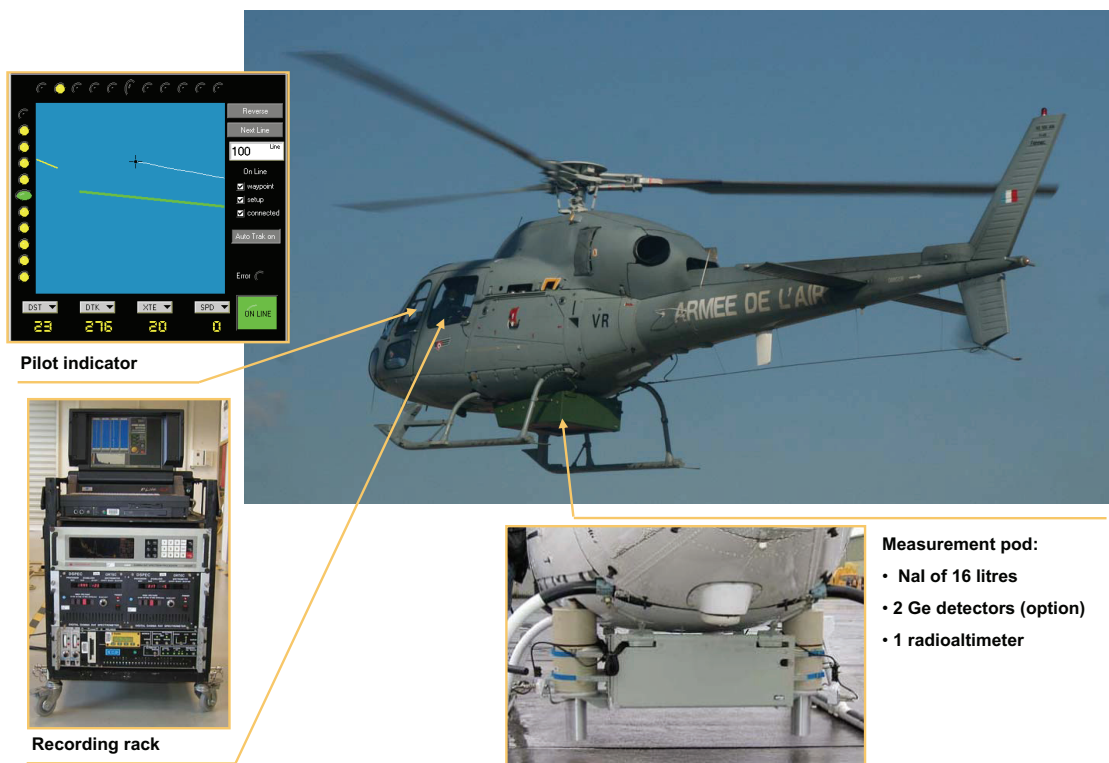
Figure 2: The French Helinuc system installed on-board an AS355 helicopter.
