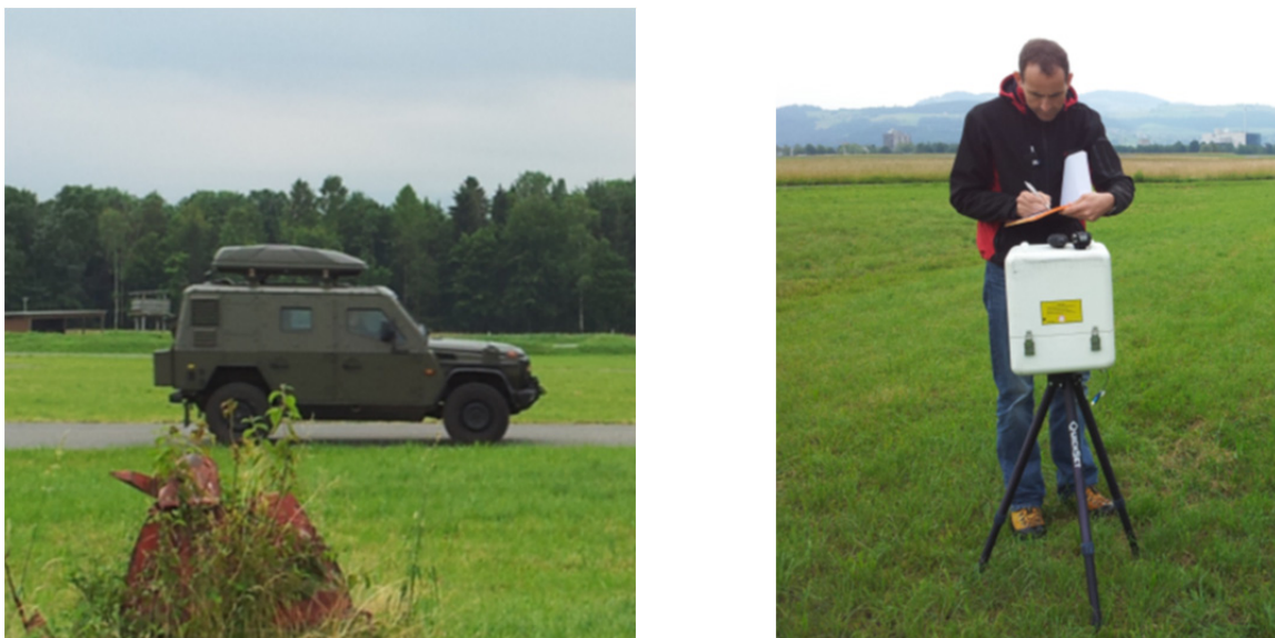
Figure 18: Vehicle equipped with gamma spectrometric equipment (left) and measurement with high pressure ionisation chamber (right).
