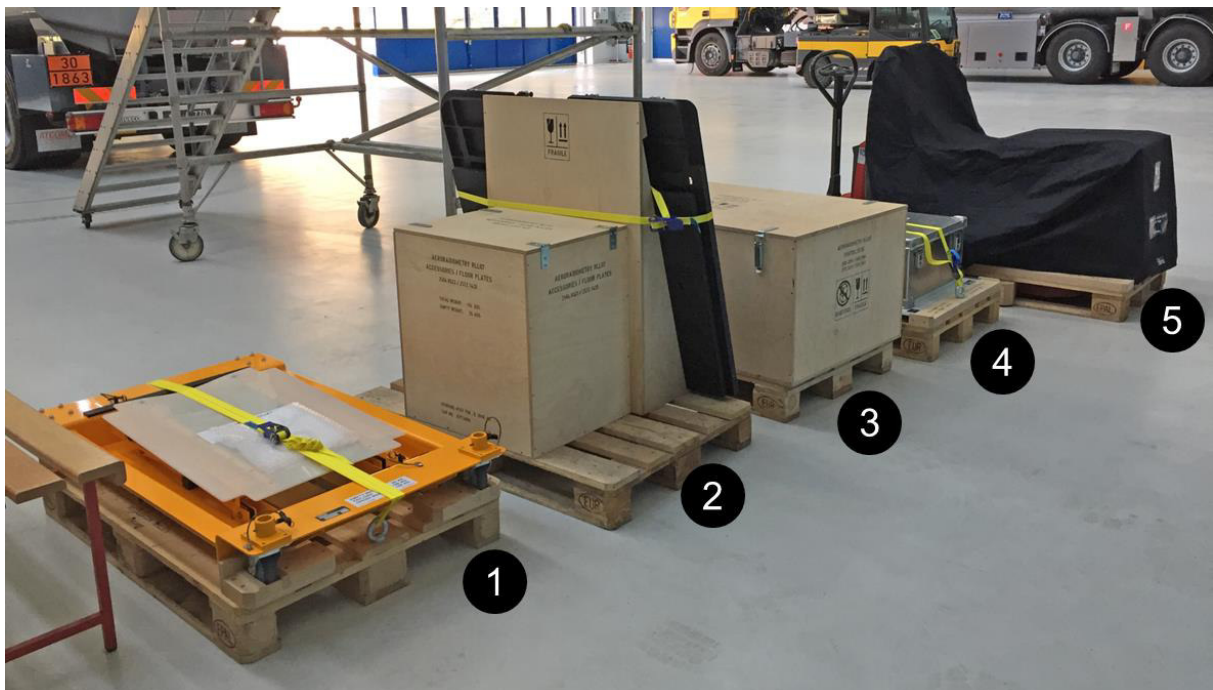
Figure 3: Components of the RLL system. 1. Lifting platform for the installation of the detection container. 2. Floor plates and accessories case. 3. Monitors and operator console. 4. Detection container. 5. Operator seats and equipment rack.
