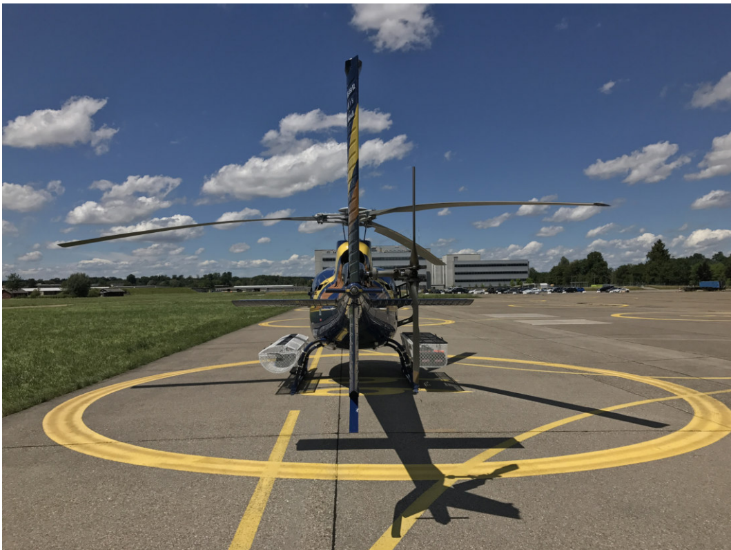
Figure 20: Rear view of the ULYSSE system installed on EUROCOPTER AS 350 B2 used during ARM17.
