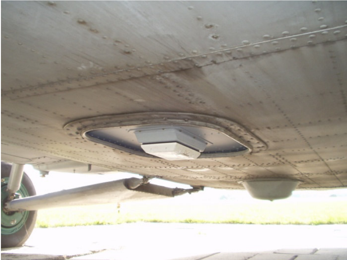
Figure 7: TR3000 radar altimeter aerial mounted below a Mi-17 helicopter.
