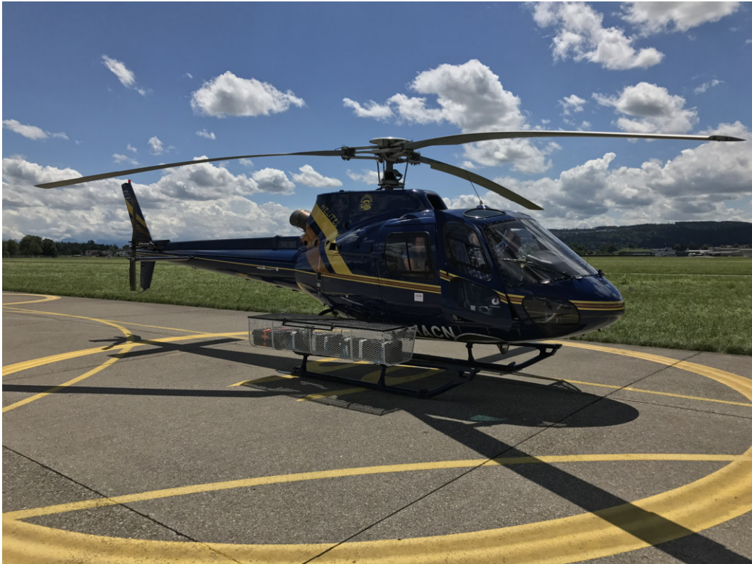
Figure 18: ULYSSE system installed on EUROCOPTER AS 350 B2 used during ARM17 viewed from the right side.
