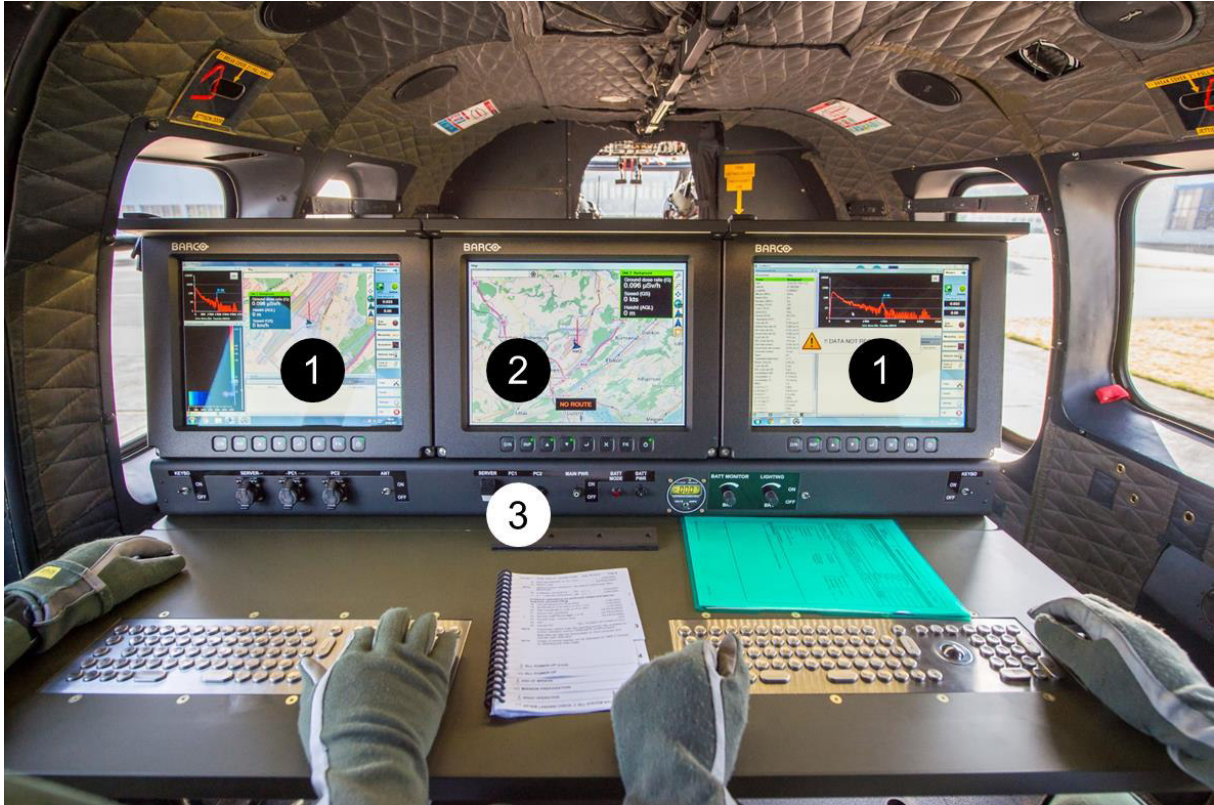
Figure 4: Operator console of the RLL system. 1. Displays of the client computers. 2. Common display (mirrored in the cockpit). 3. Control panel with switches for power, lighting and communication and USB ports for file exchange.
