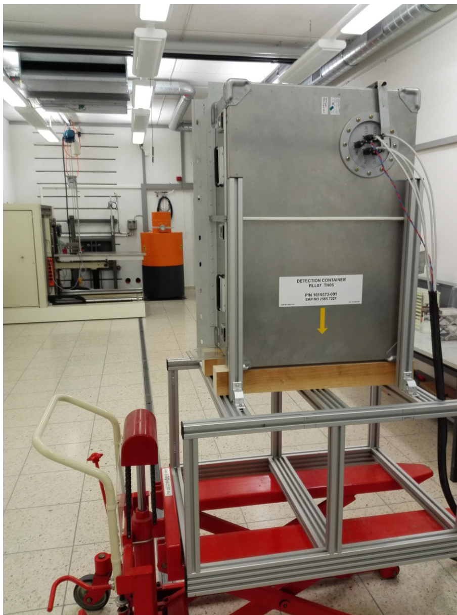
Figure 24: RLL detector 002 in the calibration laboratory at PSI.
