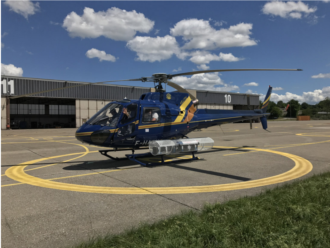
Figure 19: ULYSSE system installed on EUROCOPTER AS 350 B2 used during ARM17 viewed from the left side.
