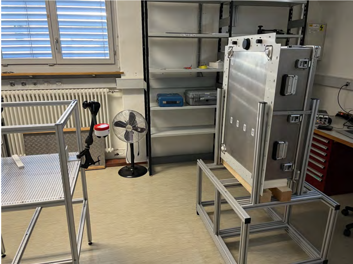
Figure 10: Detector RLL003 mounted in the laboratory for the determination of stripping factors.
