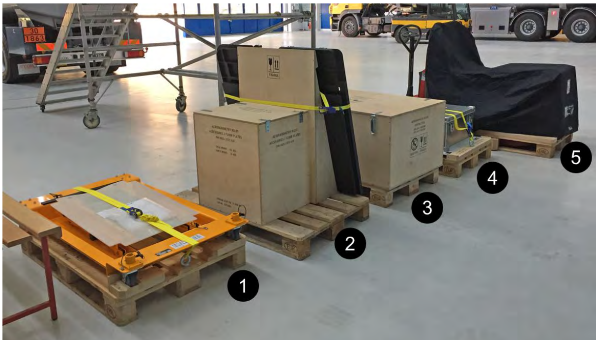
Figure 1: Components of the RLL system. 1. Lifting platform for the installation of the detection container. 2. Floor plates and accessories case. 3. Monitors and operator console. 4. Detection container. 5. Operator seats and equipment rack.
