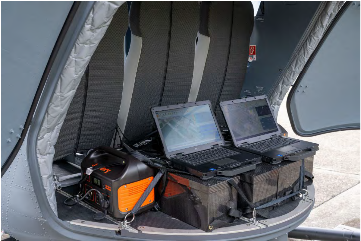
Figure 3.11: Installation of the Lithuanian aerial measurement system in the H145 helicopter.
