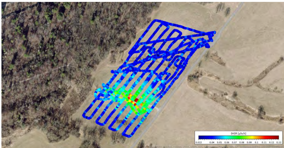
Figure 8.186: Ambient dose equivalent rate at the detector (DHSR_loc) during the drone mission, measured in Area 2 by the CZE team.
