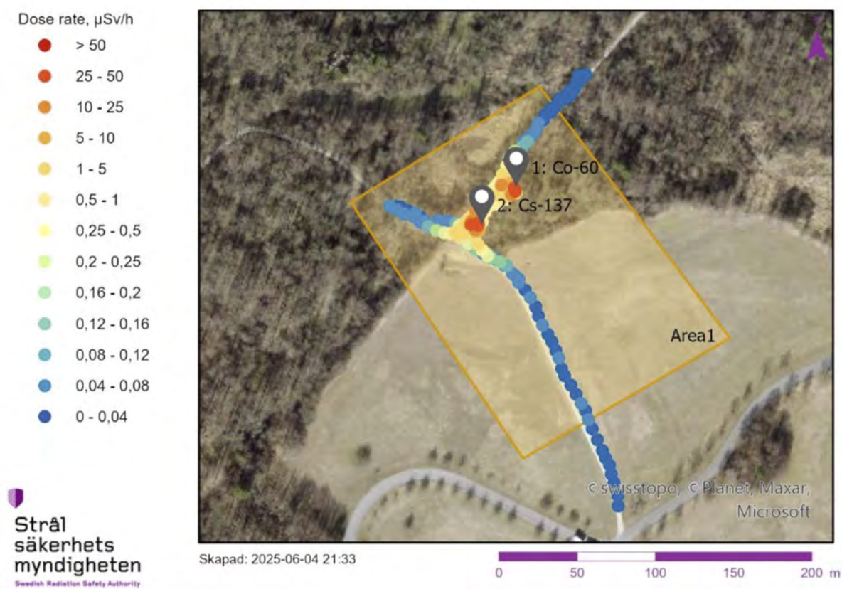
Figure 8.200: Ground-based survey results from Area 1, performed in Frauenfeld by the SWE team.
