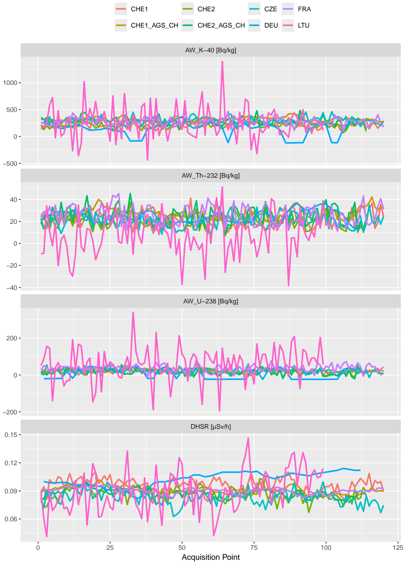
Figure 8.104: Results obtained along the common flight line flown by all teams during the composite mapping.
