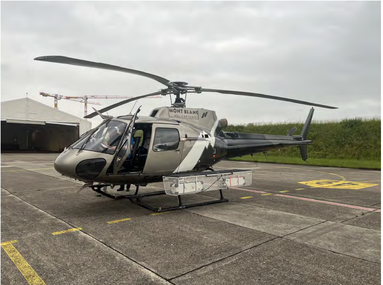
Figure 3.4: French ULYSSE system installed on EUROCOPTER AS 350 B2 used during AGC25 viewed from the right side.
