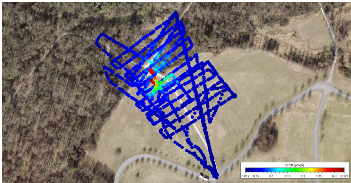
Figure 8.184: Ambient dose equivalent rate at the detector (DHSR_loc) during the drone mission, measured in Area 1 by the CZE team.
