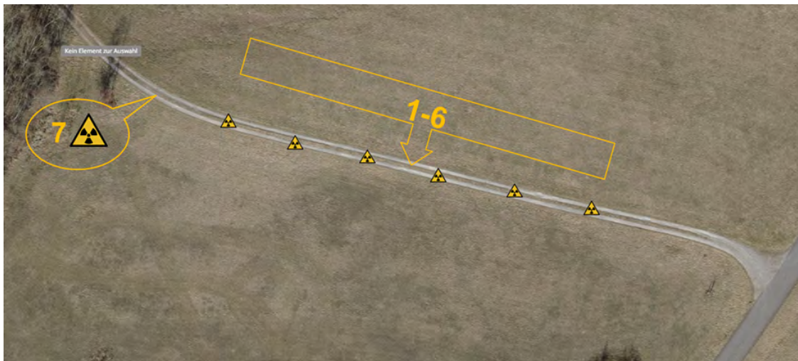
Figure 7.13: A close-up of the radioactive sources' location during Mission with Drones in Area 2.
