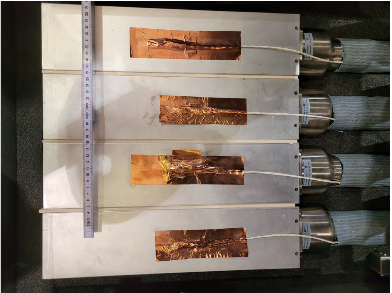
Figure 3.13: RLL Detector: 4 NaI(Tl) scintillation crystals, total volume of 16.8 L.
