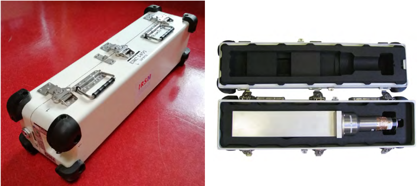
Figure 3.5: Left: IP65 box containing the 4 L NaI-detector of the ULYSSE system. Right: view of the detector components inside the IP65 box.
