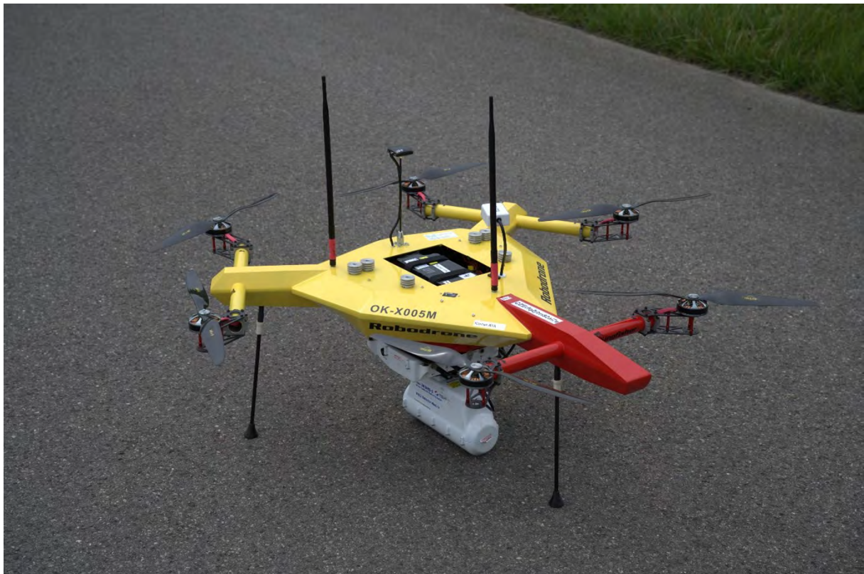
Figure 3.17: CZE Robodrone Kingfisher UAV and the base station and DRONES G by NUVIATech Instruments modular gamma spectroscopy system.
