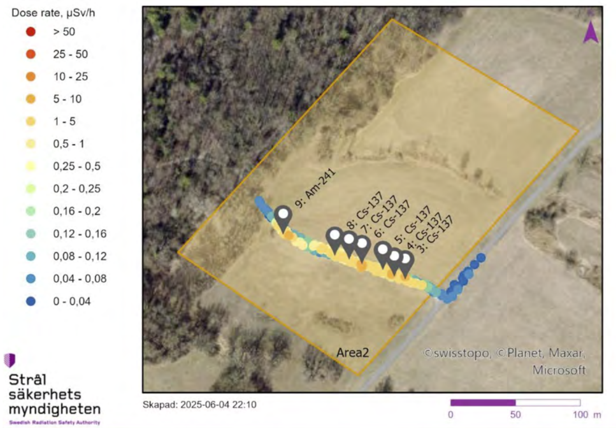
Figure 8.201: Ground-based survey results from Area 2, performed in Frauenfeld by the SWE team.
