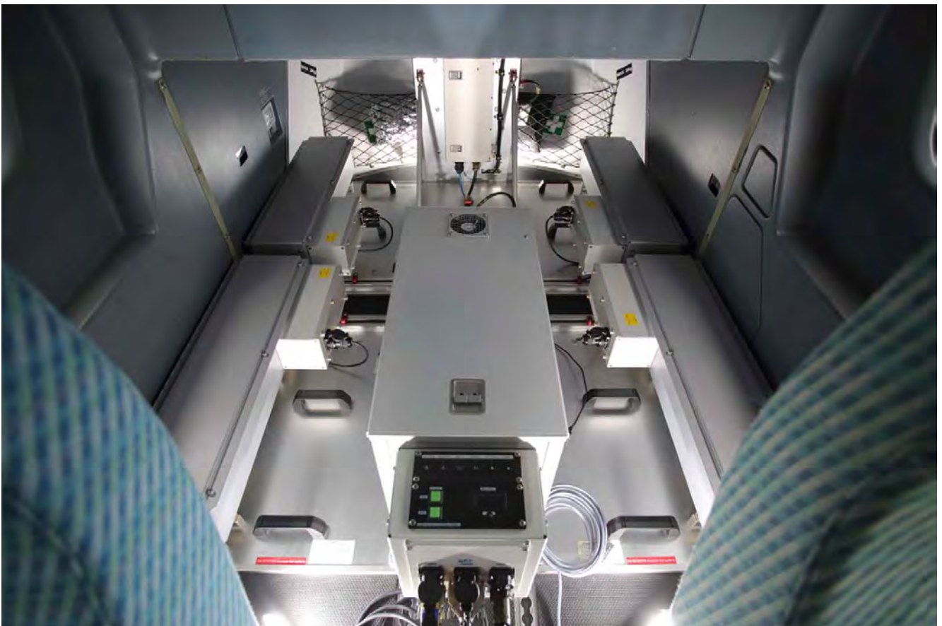
Figure 3.8: Airborne measurement system of the German Federal Office for Radiation Protection mounted in a German Federal Police type EC135 helicopter.
