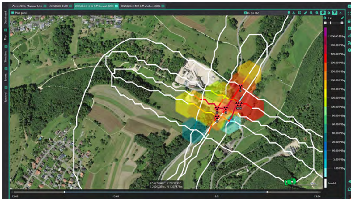
Figure 8.77: Live detection data for ^{137}\text{Cs} recorded during Mission 3 at Seebru by CHE1 team.
