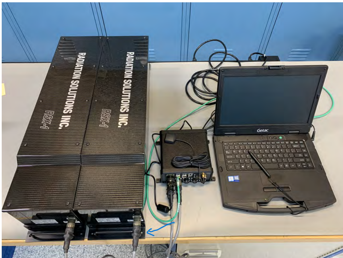
Figure 3.10: Detector package of the Lithuanian aerial measurement system (RSX1, 2 L NaI(Tl) scintillation detectors).
