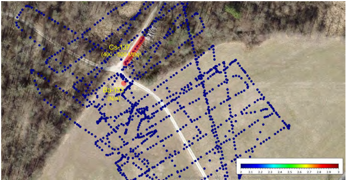
Figure 8.187: Estimation of the sources during the drone mission, measured in Area 1 by the CZE team.
