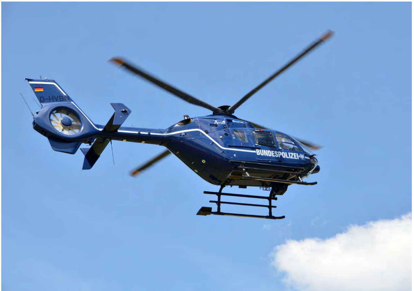
Figure 3.7: German Federal Police type EC135 helicopter used for airborne gamma-spectrometric measurements.
